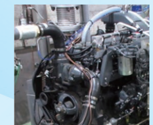
Hydrogen and diesel co-firing engine
